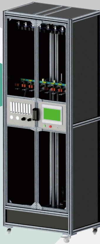
CLS2000 Catheter Laminator With 8 Stations, Re-deigned From CLS1000
