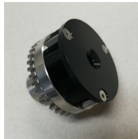
Multi-slot 6 segmented chuck, 0-1/4" opening, plastic segments, directly hold tubing and/or mandrel, easy loading/unloading. No calibration needed
