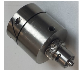
Luer lock chuck can hold and rotate a catheter with pre-molded luer
